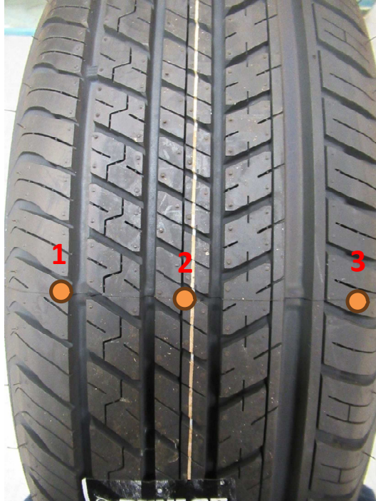
Figure 25. Measurement procedure - Measure points shore A hardness
