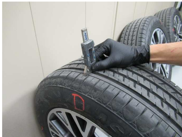
Figure 24. Measurement procedure - Measure tread depth of main grooves
