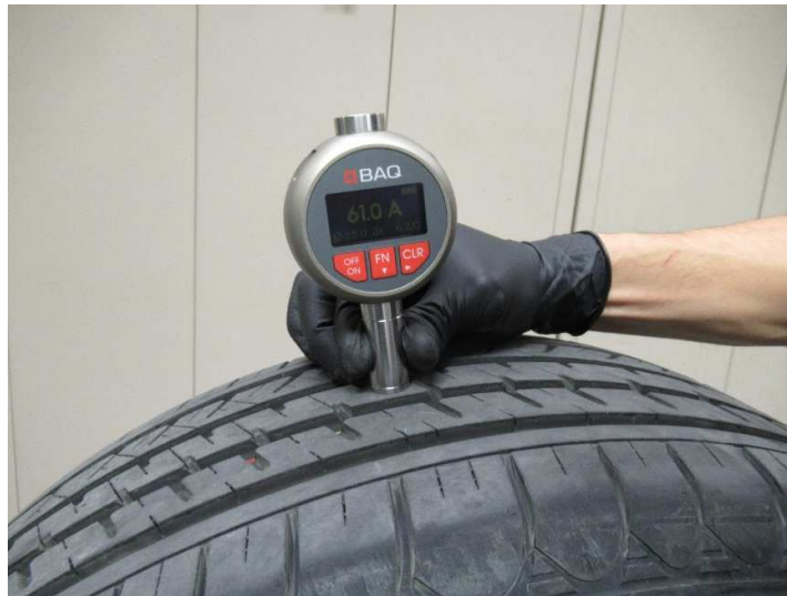
Figure 26. Measurement procedure - Measure shore A hardness
