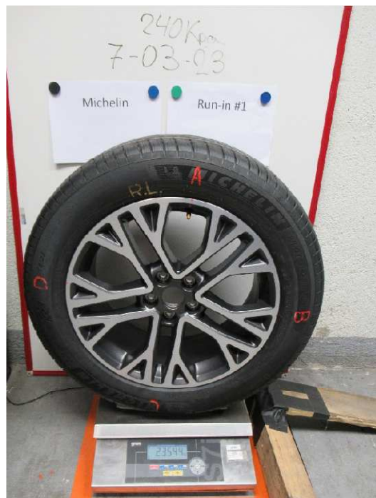
Figure 20. Measurement procedure - Weight measurement.
