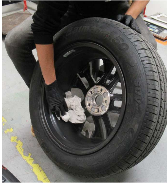
Figure 19. Measurement procedure - Clean the rim surfaces.
