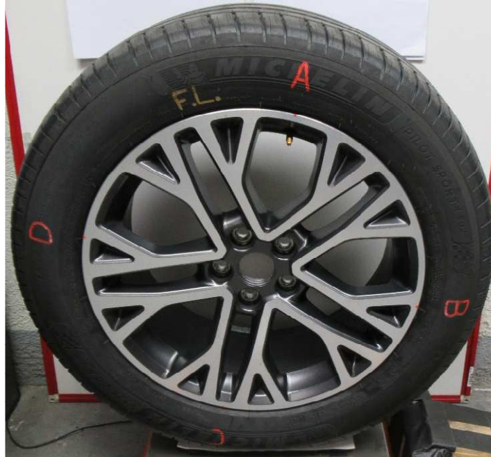
Figure 23. Measurement procedure - Mark the tyre in four places every 90°
