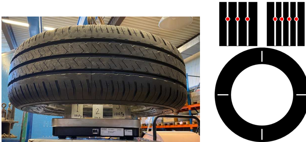
Figure 151. Right: Weighing of tyre with rim. Left: Tread depth measurement positions on the tyre and on the tread depending on 3 or 4 longitudinal grooves.
