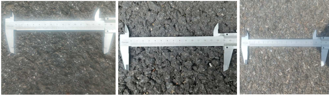
Figure 132. Road surface characteristics (urban, rural, motorway).
