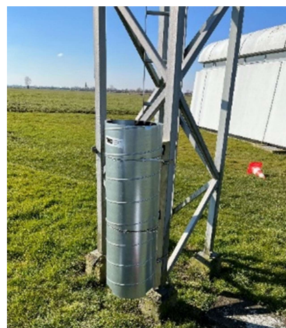
Figure 8 Total deposition sampler at Cabauw
