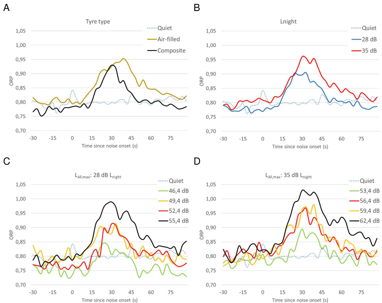
Figure 14 Event-related change in Odds Ratio Product (ORP). Data are arithmetic means across all subjects and noise events, stratified by type of tyre (panel A ), L_{night} (panel B ), and L_{AF,max} (panels C and D ). Data for the Quiet condition are derived from data in the Control night at clock times corresponding to the timing of events in the noise nights.
