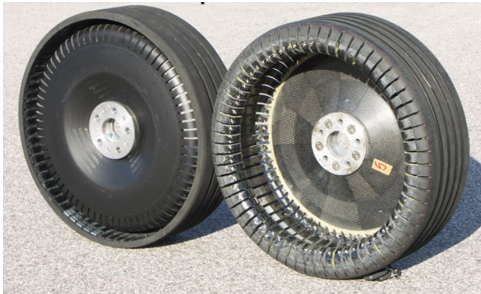
Figure 5: The airless tyre (Composite Wheel) final prototypes produced in the international project 2003-2008. The left part shows the outside of the tyre; the right part shows the inside (to be mounted towards the car chassis). Not shown here are the small holes (diameter 7 mm) drilled in the bottom of the grooves in the rubber tread.
