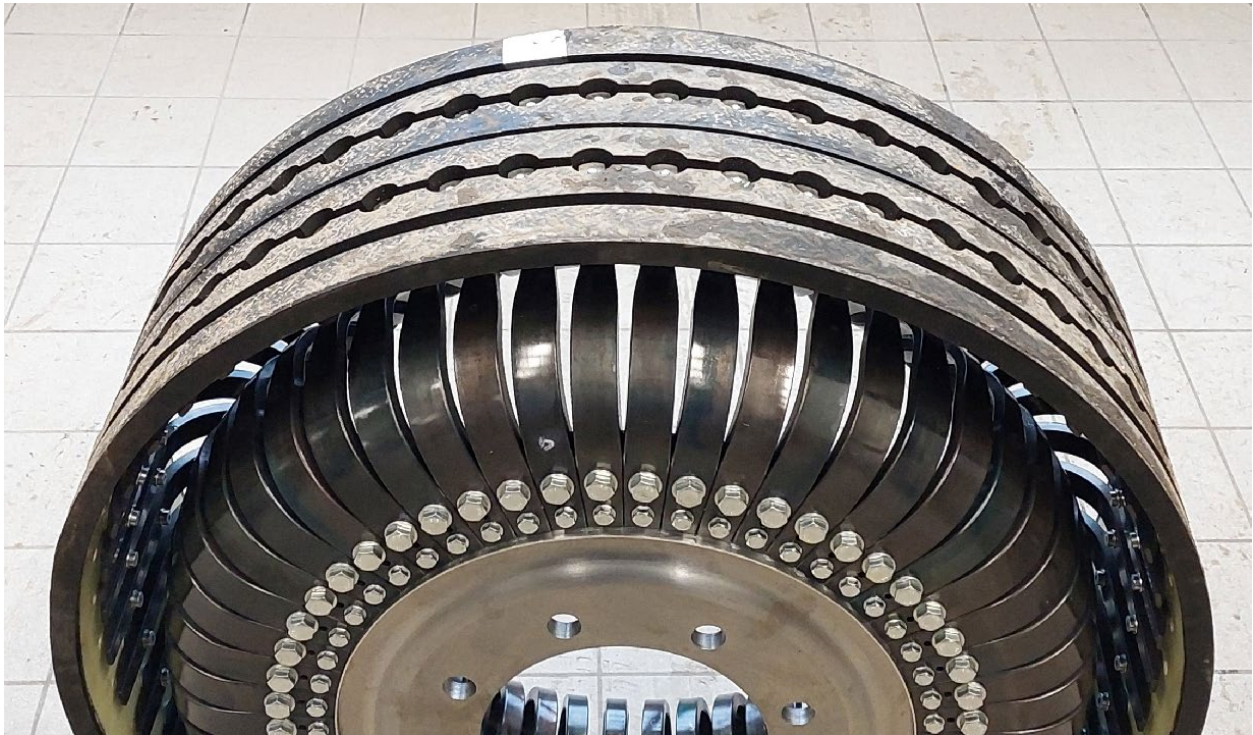
Figure 11: The first physical prototype shown at an angle where the rubber tread can be seen. Note that two wider grooves include bolts to connect the belt to the spokes.
