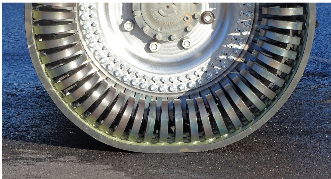
Figure 14: A closer view of the deflection of the spokes in the contact patch for a static load of approx. 2000 kg.
