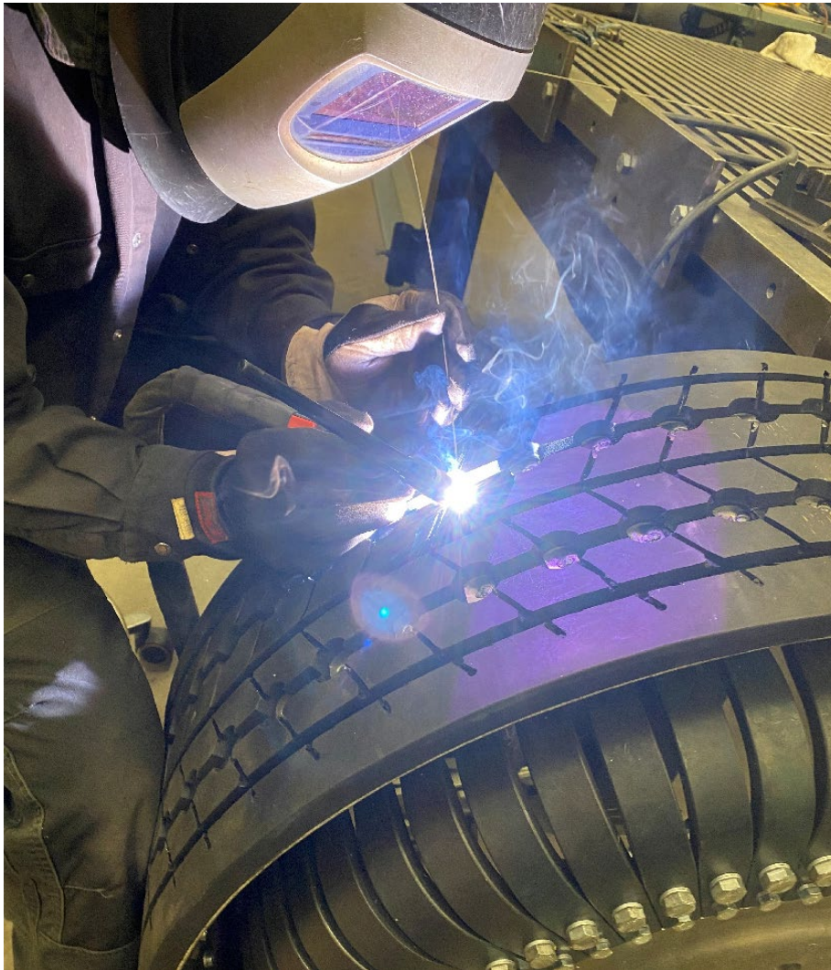
Figure 27: Welding of nuts on the bolts, made by the VTI welding specialist, to secure that they cannot separate during the tests.
