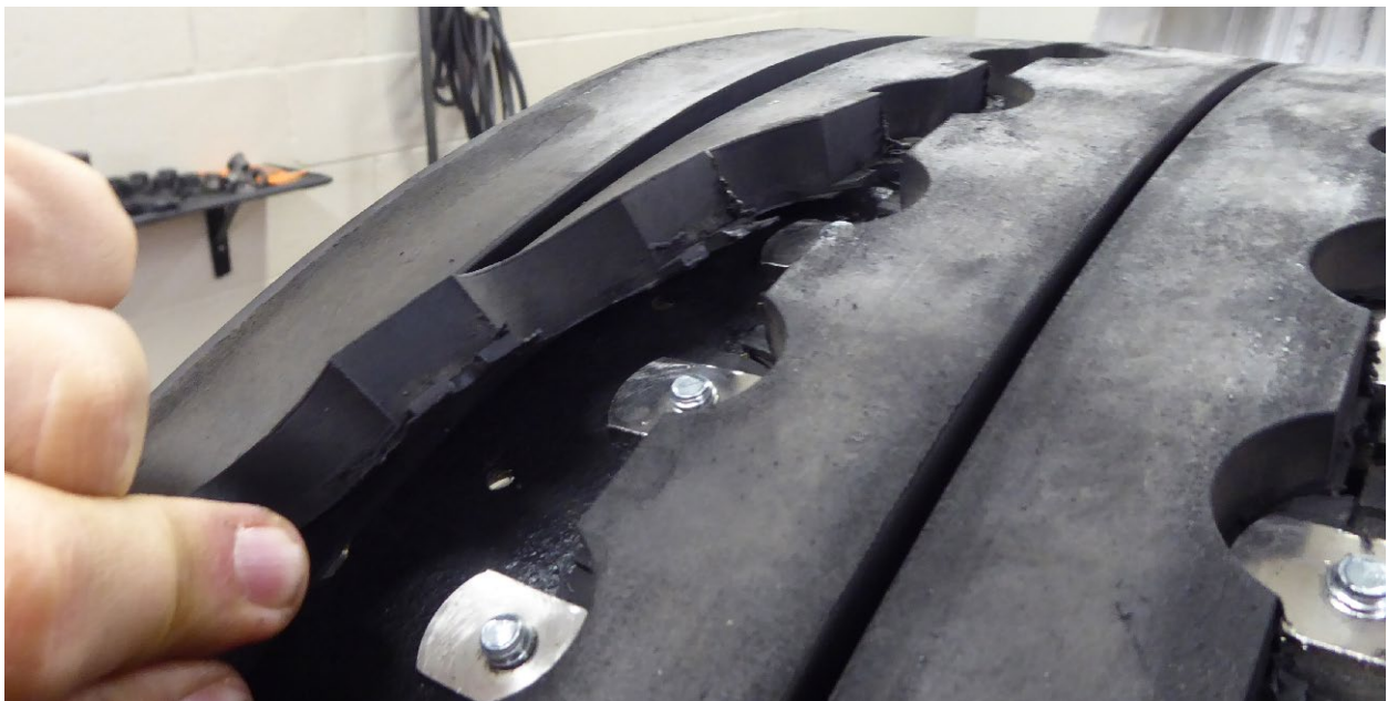
Figure 22: An example of how the rubber tread had separated from the CFRP belt. This happened at several places along the tread.
