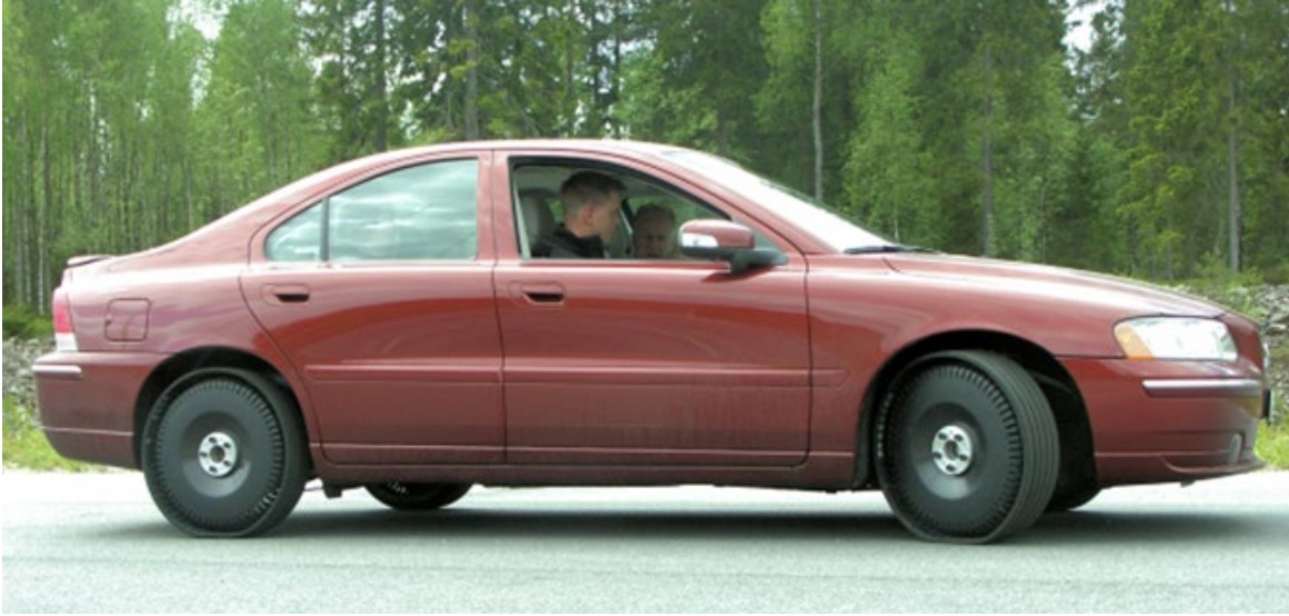
Figure 4: The Composite Wheels mounted on a Volvo car for various tests in 2008. Photo by the author.
