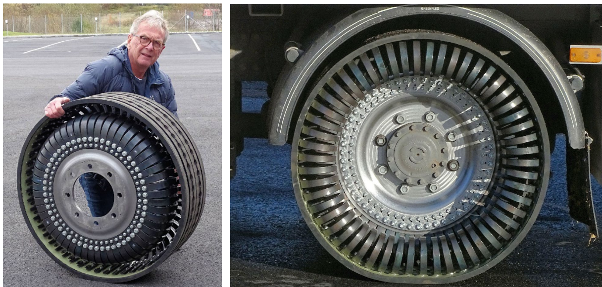
Figure 1: The first prototype for an airless tyre, for use on steering and trailer axles of a heavy goods vehicle (HGV). The left photo also shows Mr Hansson; the inventor.
