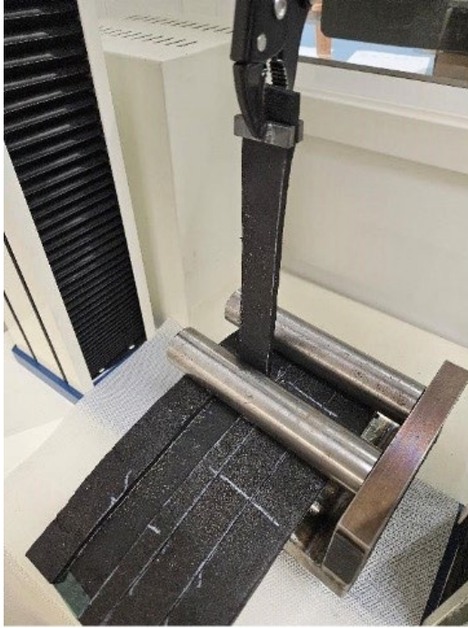
Figure 23: Simple setup of a test to measure the available tensile stresses between belt and rubber before separation. The material samples in the picture are from another project.
