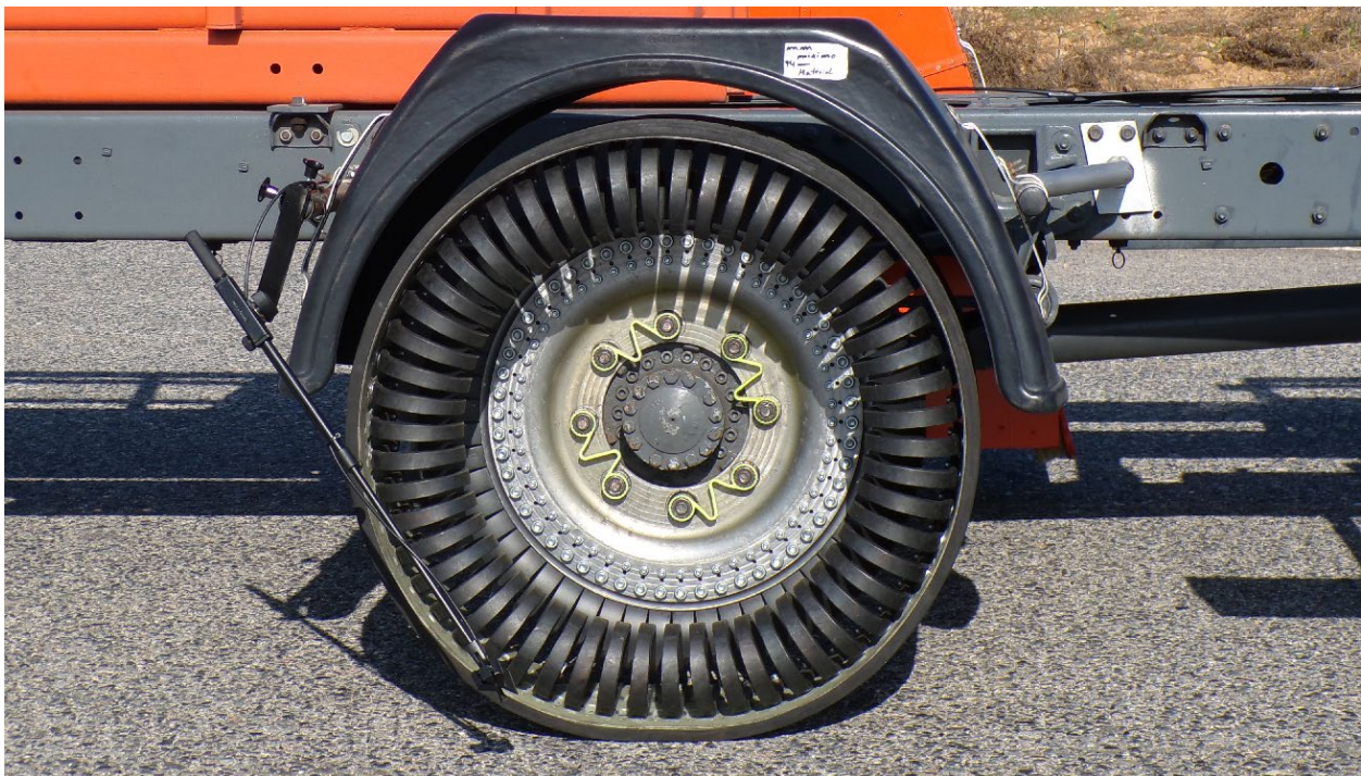
Figure 22: The airless tyre prototype 1b mounted on the test truck for noise measurements. Microphone holder is shown but the microphone itself was not mounted on this picture.
